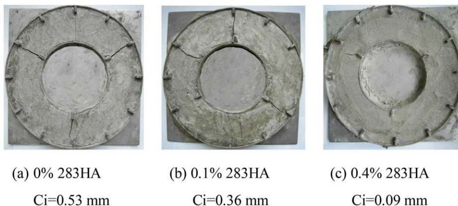
Figure 7. Crack tendency of cement pastes with (a) 0%, (b) 0.1%, and (c) 0.4% 283HA after 1-day air blowing. [Color figure can be viewed in the online issue, which is available at wileyonlinelibrary.com .]
